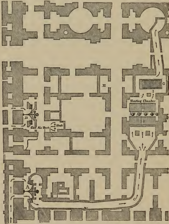
FIGURE 28.—PLAN SHOWING AIR DUCTS, ETC., IN CONNECTION WITH HEATING APPARATUS, SOUTH WING, U. S. CAPITOL.
